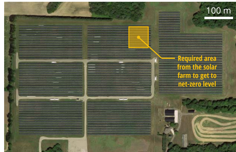
Figure 11: The area of off-site generation required by the development (yellow rectangle) overlaid on the Silvercreek Solar Park, found near Aylmer Ontario (image Courtesy of Google Earth™).
